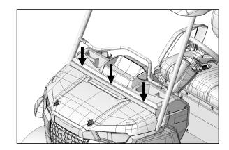
• Lay the windshield assembly (1) against the A-pillars.
