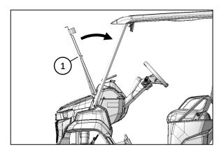
• Fasten the top half of the windshield assembly (1) to the A-pillars with the rubber hooks.
