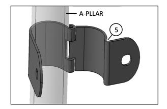
Close clamp around A-pillar and secure with sockethead bolt (3), washer (4) and rubber damper (7) as shown.
