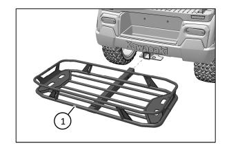
• Line up the cargo rack holes with the hitch receiver holes and install hitch pin (#TLR39) as shown.
